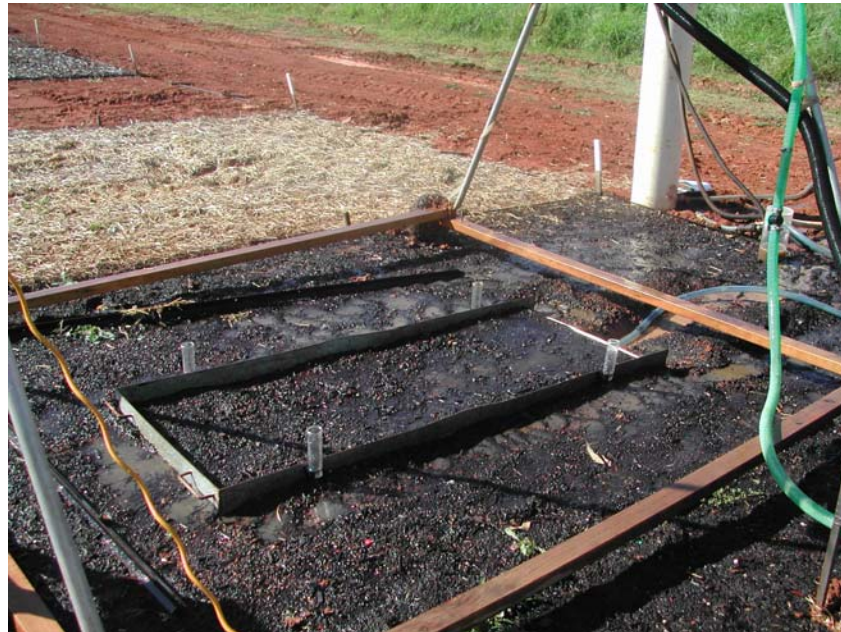
Figure 4: The rainfall simulation plot area (as hemmed in by the 3-sided metal guard, with the collection tray at the front end of the plot)
