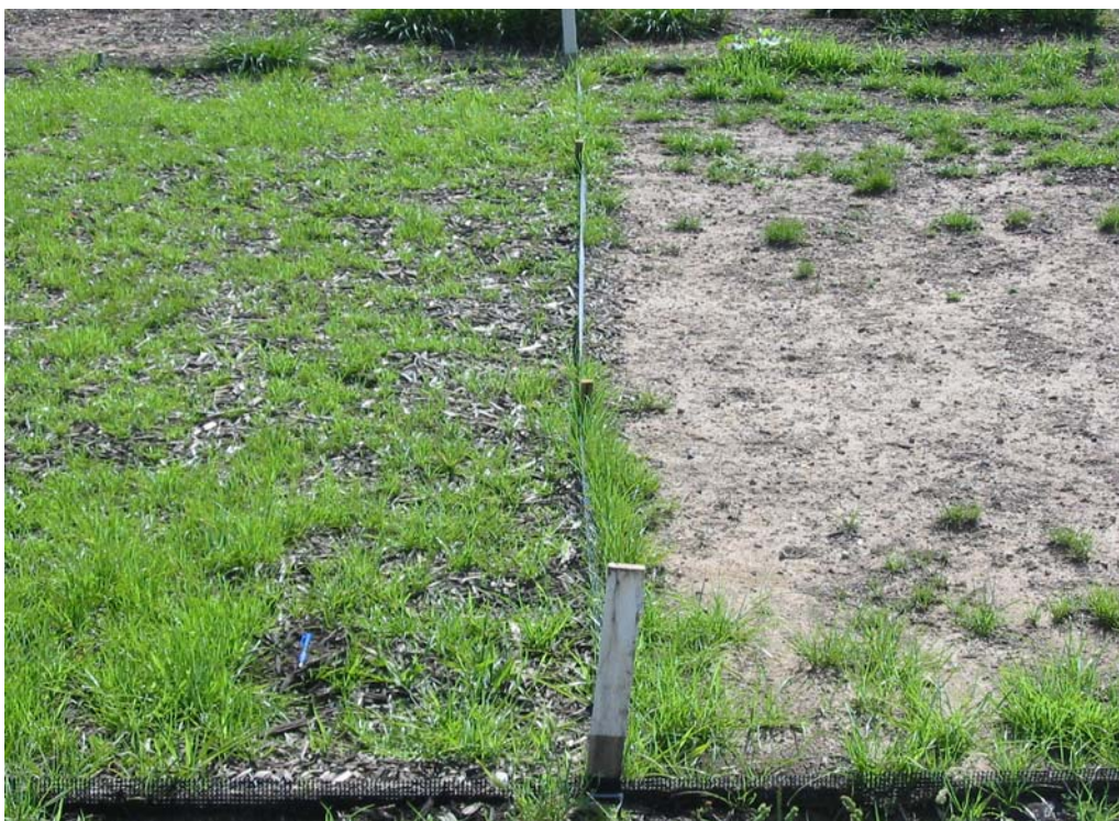
Figure 33: Vegetation cover on a mulch plot (left) and a soil conditioner plot (right) at the Bungonia trial site
